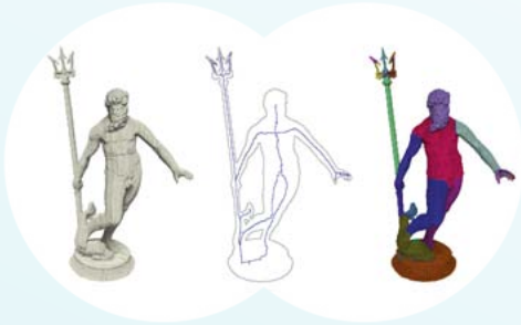
Automatic decomposition (on the right) of a shape (on the left) using a curvilinear skeleton (middle) (John Chaussard)
